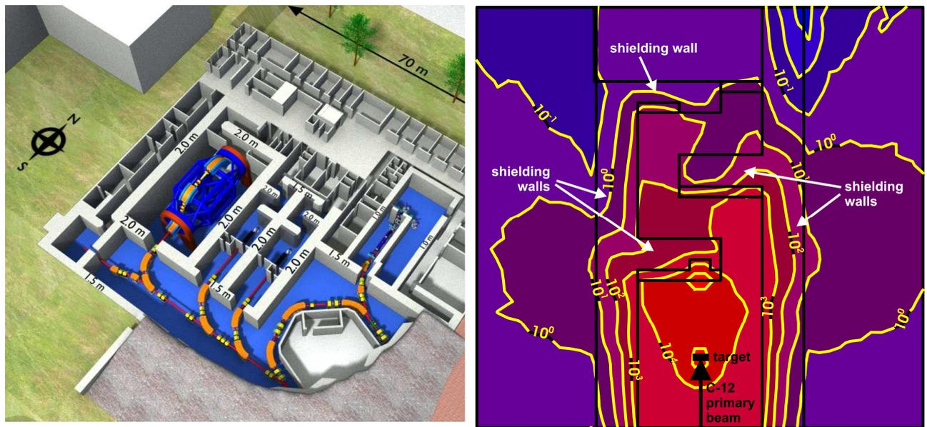
2659 Figure 3.27. Left: Part of the HIT facility in Heidelberg. Right: The dose distribution in the horizontal
