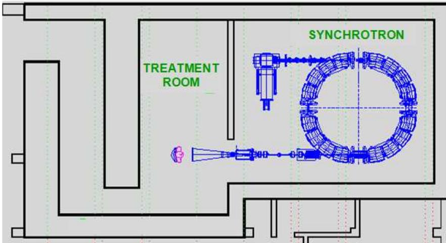
1498 Figure 2.16. Schematic layout of single-room synchrotron-based proton therapy system (Courtesy of
