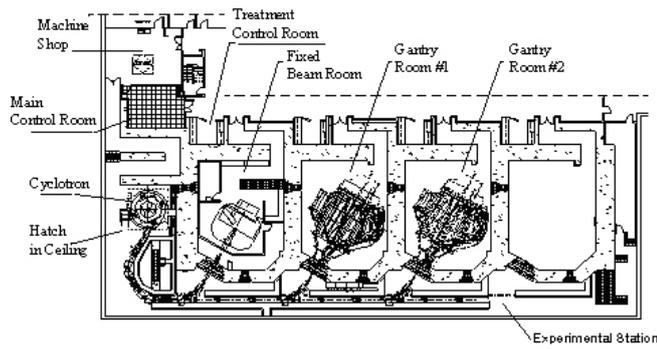
Fig. 1. Layout of proton therapy part of the building showing treatment rooms, cyclotron and beamlines.
