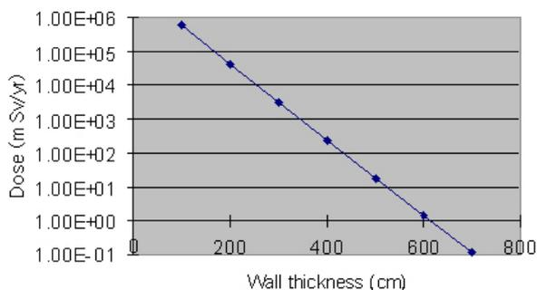
Fig. 6. Dose output of the shielding wall near the ESS region facing the parking lot versus concrete-equivalent wall thickness.
