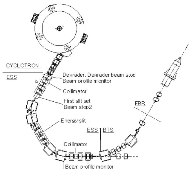
Fig. 5. Major locations of proton beam losses in the ESS area.
