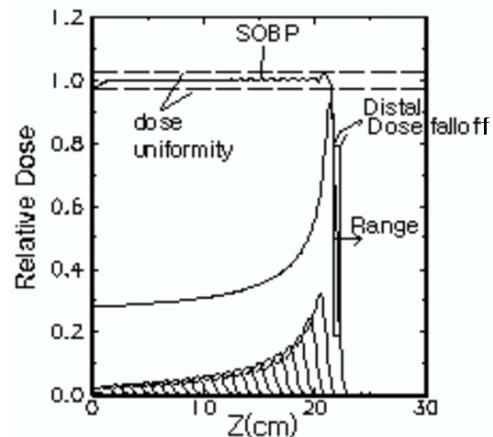
Fig. 4. Definition of SOBP, beam range, distal dose falloff, and dose uniformity.
