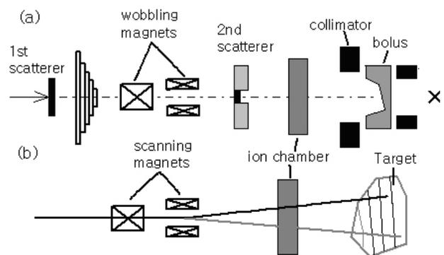
Fig. 3. (a) IBA nozzle to perform both single or double scattering and wobbling. (b) Pencil Beam Scanning nozzle.
