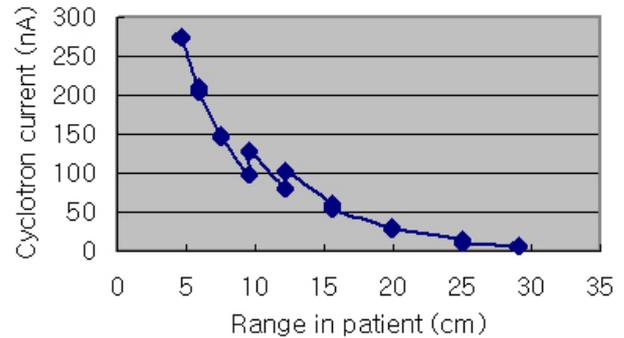
Fig. 2. Cyclotron current as a function of proton range in patient at a dose rate of 2 Gy/min.
