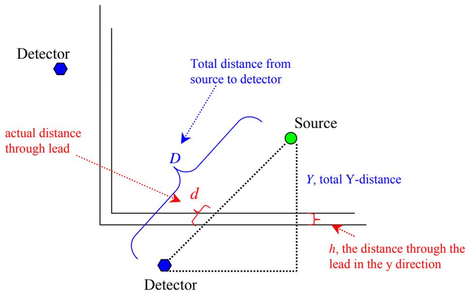
**Fig. 11:** Illustration of source to detector geometry
