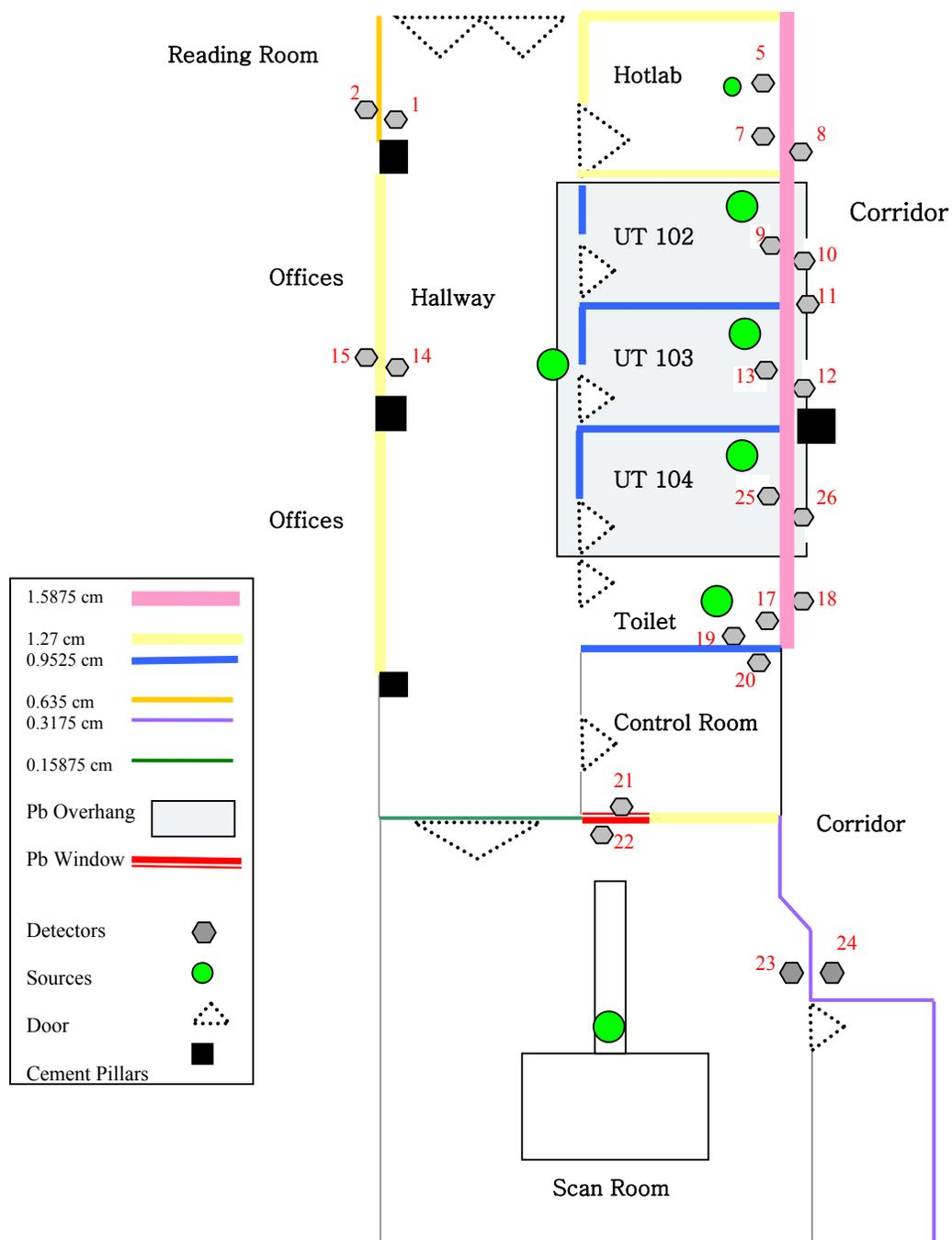
**Fig. 9:** The location of sources and detectors within the PET/CT suite (detectors 3, 4, & 6, not used)
