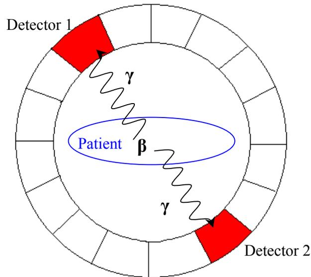
**Fig. 4:** How photons are detected in PET
