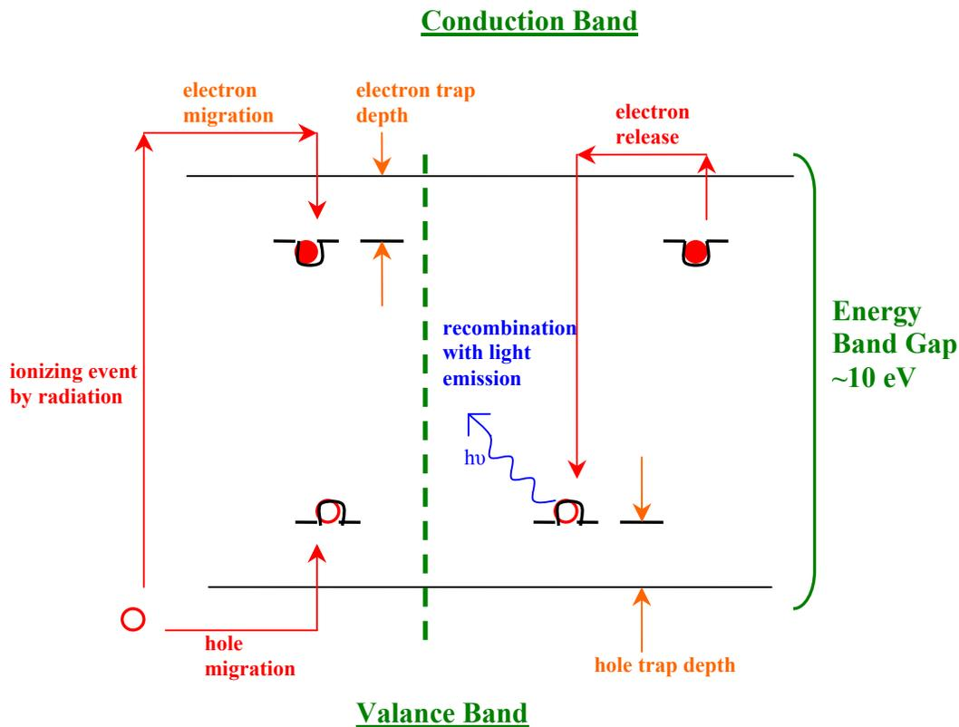
Fig. 5: A representation of the luminescence (Attix 2004)
