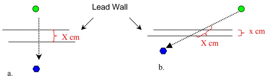
**Fig. 12:** a. Effective thickness of lead slab; b. Same effective thickness with different actual thickness
